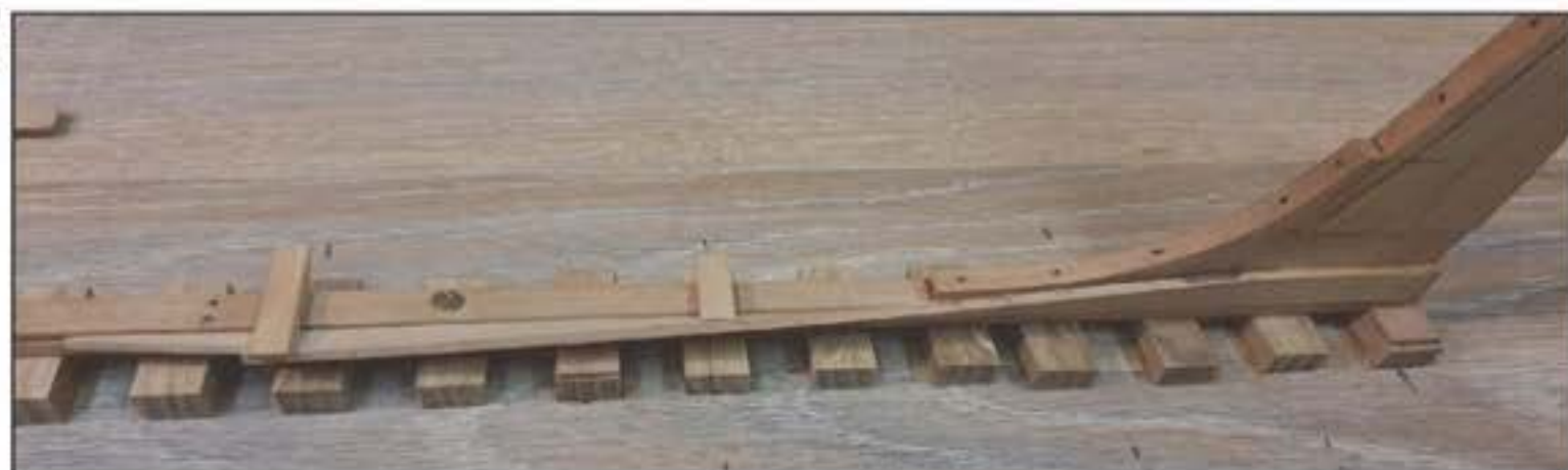
8. A twisting garboard strake modeled by Maarten Bunte. The position of the plank changes from almost horizontal to vertical against the stem. The location of the rotation determines the shape of the hull.
